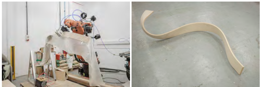
Fig. 1.9: Free-form optically-guided vacuum lamination with Jonny Martin (2015).
