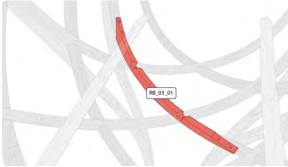
(a) A single rib element, annotated as RB_{03\_01} : where RB signifies rib , 03 denotes the third grid line, and 01 denotes the second segment of the grid line.
