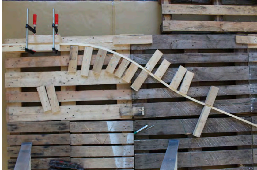
Fig. 5.2: The bending performance and elastica of the 20 x 20 mm lamella are explored intuitively in Probe 2: IBT glulam workshop .
