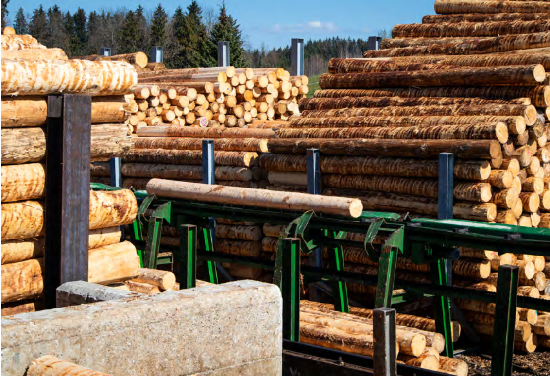
Fig. 3.9: Incoming logs at the Blumer Lehmann AG sawmill are sorted according to diameter.
