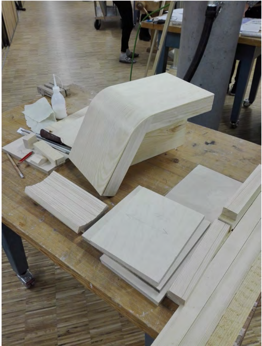
Fig. 5.24: The cross-laminated material prototype of Prototype 4: Slussen benches with the laminated skin.
