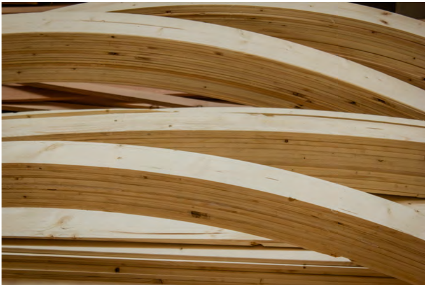
Fig. 6.53: The finished glulam blanks awaiting machining.
