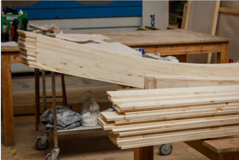
Fig. 6.49: The sawn spruce lamellae and a finished glulam blank.
