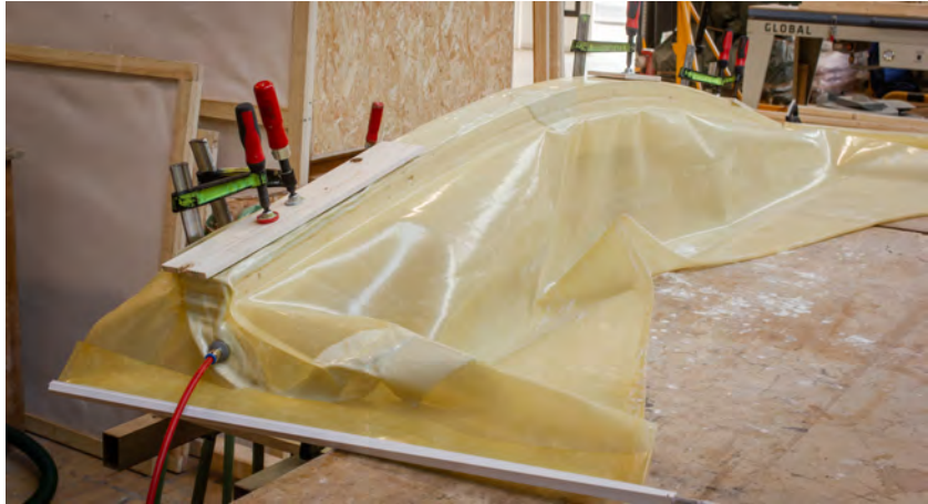
Fig. 6.50: The pressing framework uses a vacuum press and minimal hand clamps.
