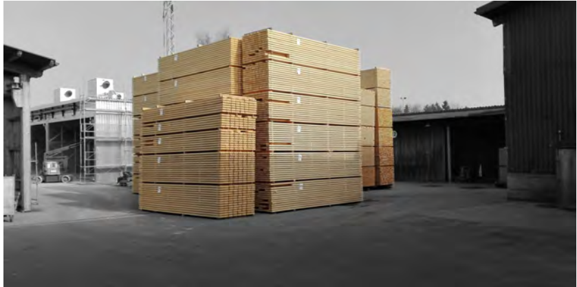
(a) Dimensioned lumber, the raw input for the production of a glulam blank.
