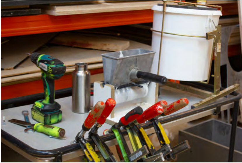
Fig. 6.51: The necessary hand tools for the pressing framework: a cordless screwdriver, glue roller, clamps, and glue.
