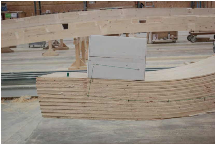
(b) Comparison of where the production data is (drawn green outline) versus where the material is.
