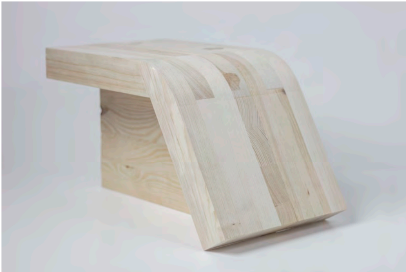
Fig. 5.23: The cross-laminated material prototype of Prototype 4: Slussen benches without the laminated skin.
