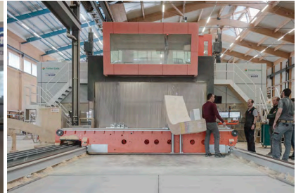
(b) The multi-axis CNC production centre at Blumer Lehmann AG .
