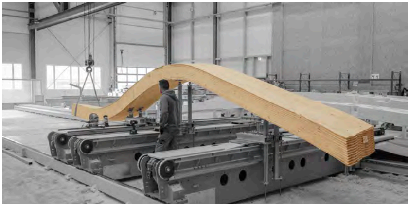
(b) The free-form glulam blank.
