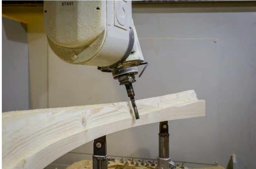
Fig. 6.52: The five-axis machining framework is more similar to the production mill at Blumer Lehmann AG than the robotic arm.
