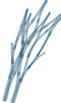
(d) Dimensioned glulam blank models including overlaps for cutting joints.
