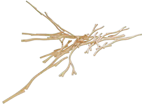
Fig. 6.5: Aggregating free-form glulam members through architectural notions of splicing, peeling, and bending.
