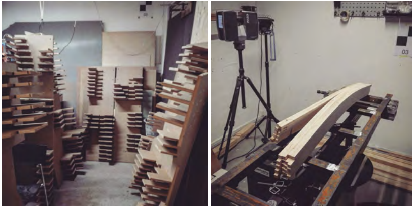
(a) Laser-cut MDF moulds used for the Probe 5: Branching Probe and Prototype 2: Grove prototypes. (b) 3D scanning the formed prototype for testing the quality.
