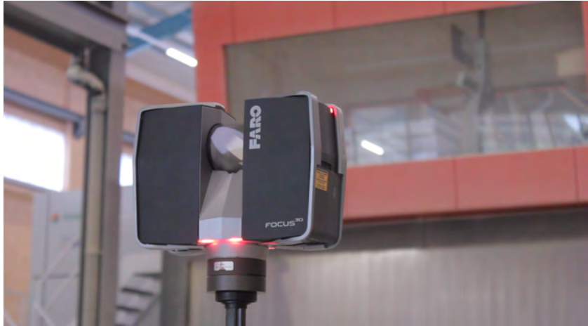
Fig. 5.41: The Faro Focus 3D LiDAR scanner in the Blumer Lehmann AG production environment.
