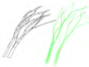
(a) The solid model of the demonstrator. (b) The accompanying glulam blank model gives feedback of material specification and lamella sizes.
