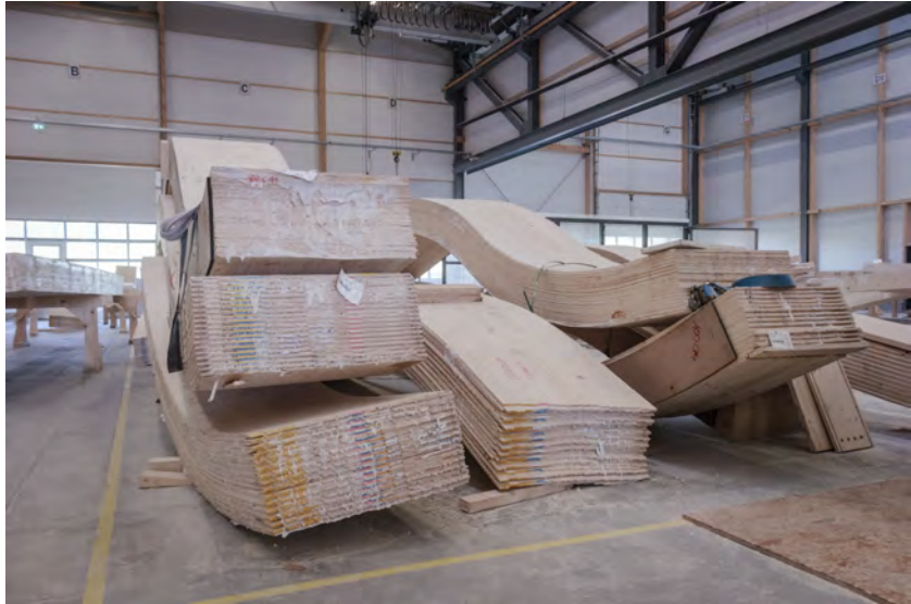
Fig. 5.29: The non-orientable free-form glulam blanks increase uncertainty and risk.
