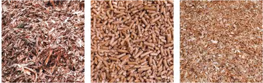
Fig. 3.11: Smaller elements of the saw milling process. Waste from the debarking process (left), compressed wood pellets ready for packaging and use as fuel (centre), and wood chip waste from the saw milling process (right).
